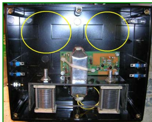
Plate capacitor tuners, silver Sephorah radio coil and solid state amplification visible pre-wiring. Yellow circles show approximate location of input and output wells.
